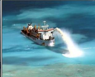
Figure 15: Tian Jing Hao, Cutter-Suction Dredge (Annex 858)
